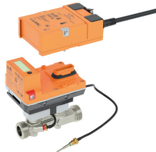
Fig. 47: All wiring is to the logic module, allowing the EN1434/MID sensor module to be recalibrated without disturbing the wiring.
